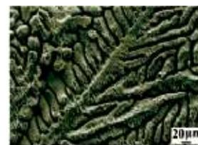
Typical corrosion morphology after 16 h of immersion (complete removal of GB phases; Mg-10Gd-6Zn alloy)
