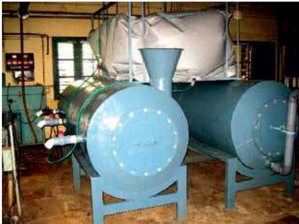
*Photograph of the anaerobic digester for biomass wastes treatment at 100kg/day*
