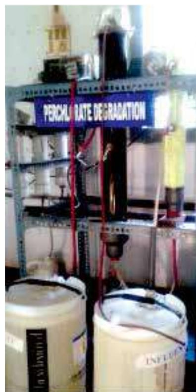
Perchlorate treating bioreactor
