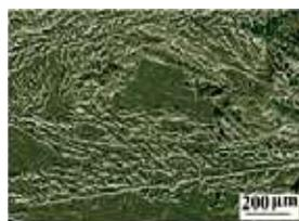
Typical filiform corrosion after 5 h of immersion (Mg-10Gd-2Zn alloy)
