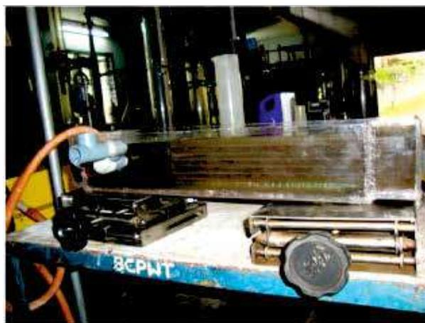
Photograph of the innovative co-current tube settler fabricated in-house at NIIST.
