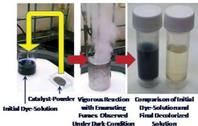
Industrial Dye-Removal via "one-stop" Dark Catalysis Mechanism using novel Flyash-based composites
