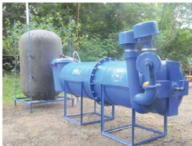
*Photograph of the commercial anaerobic treatment system cum biogas plant for household biodegradable wastes*
