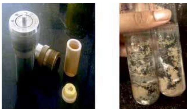
Fig 12 A-Catalytic biomass hydrolysis being performed in acid digestion bombs, B-mixture of biomass and catalyst
