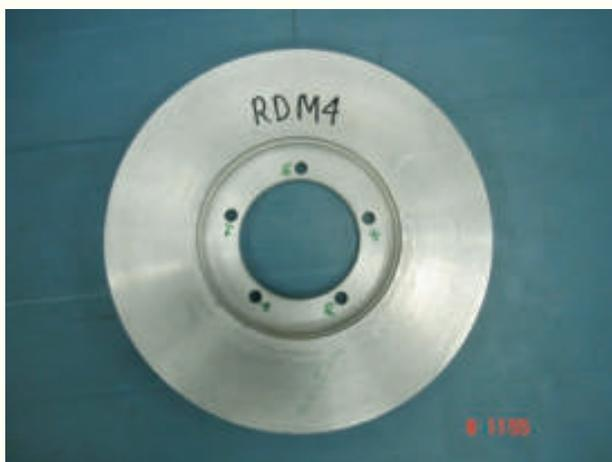
*Al-SiC functionally graded prototype brake rotor disc*
