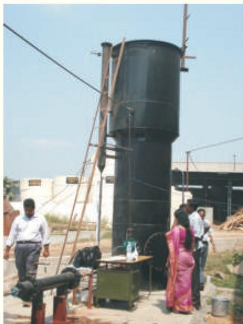
UASB reactor for parboil effluent treatment pilot plant
