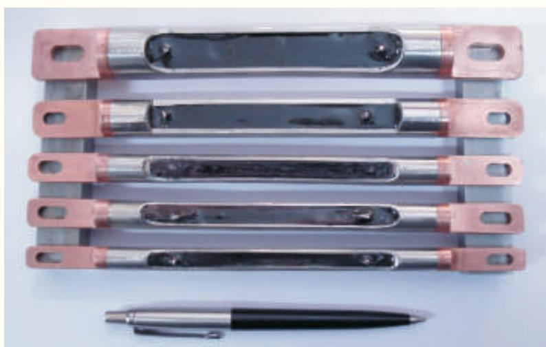
*The superconducting current leads developed by NIIST in collaboration with RRCAT
