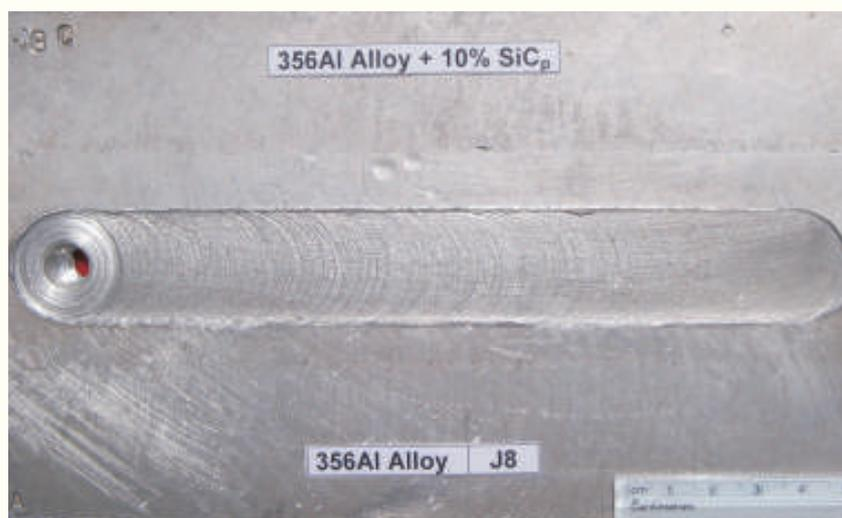
*356Al - 356Al/10% SiCp plates joined by friction stir welding.*
