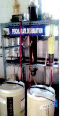
Perchlorate treating bioreactor
