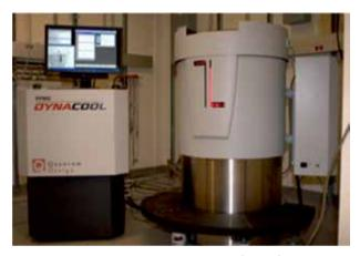
Quantum Design – Cryogen Free Physical Property Measurement System
