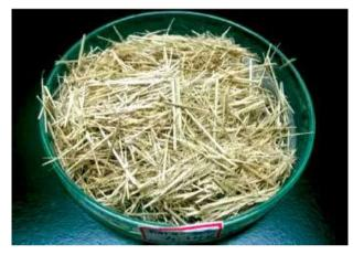
Clean fibres extracted by high solids anaerobic processing
