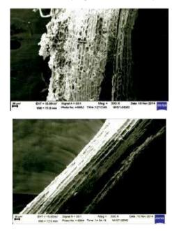
Electron micrographs of coconut leafstalk fibre before and after anaerobic treatment
