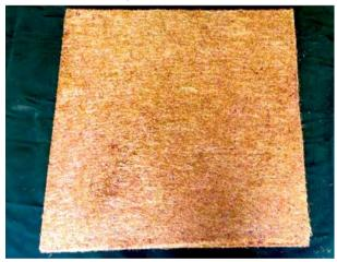
Photograph of the coir composite panel developed for acoustic application
