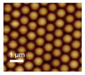
Atomic force micrograph showing the self-assembling of SiO<sub>2</sub> nano spheres
