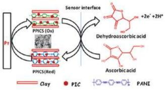
Schematic representation of the proposed PPICS modified platinum electrode and its electrochemical reaction with ascorbic acid
