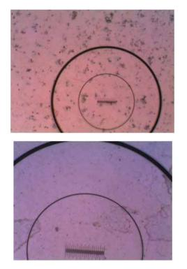
Coated paper. top: clay before flotation; below: clay after flotation; bar 0.1 mm;
