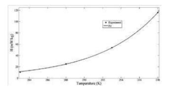
Figure: Exponential variation of heat generation due to degradation with temperature.
