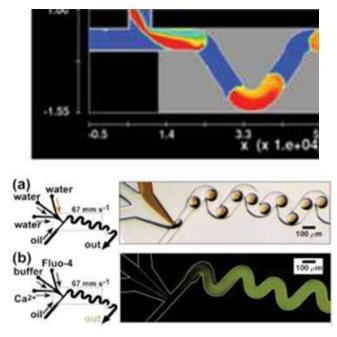
Contour plot of concentration of reagent A along with the experimental results
