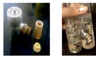
Fig 12 A-Catalytic biomass hydrolysis being performed in acid digestion bombs, B-mixture of biomass and catalyst
