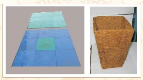
Roof tiles based on coir - rubber composites. Garden pot based on coir-sheet
