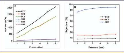
(A) Graph of flux measurement on uncoated tube (UCT), intermediate alumina coated tube-1 (SCT) and tube-2 (SCT) and final  $TiO_2$  coat on slurry-boehmite coated on tube-1 (SBT), tube-2 and tube-3 (repeated on 3 tubes), (B) Rejection (%) of BSA against pressure, UCT uncoated tube, S-CT Precoated alumina tube, SBT- Precoat and final coat tube.
