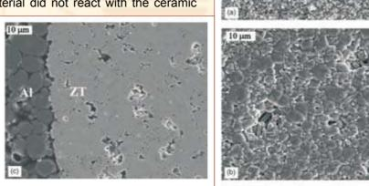
Surface morphology of (a) green  $Zn_2Te_3O_8+4$  wt% TiO<sub>2</sub> tape (b) Tape sintered at 660°C (c) cross sectional view of the interface between Al electrode and the tape sintered at 660°C indicating non-reactivity.
