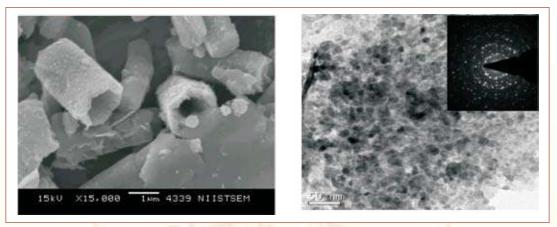
SEM and HRTEM images of ZnO microtube and ultrasonicated nano-ZnO particles
