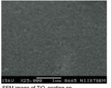
SEM image of TiO<sub>2</sub> coating on glazed tile calcined at 700°C
