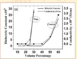
Variation of relative permittivity and conductivity as a function of volume % of filler for fine and coarse filler particles
