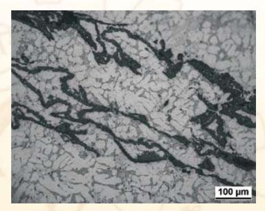
Optical micrograph of the in-situ AI-7Si-0.3Mg (356)-4Mg-AIN composite after 4 hours reaction (gas flow rate: 0.4lpm)
