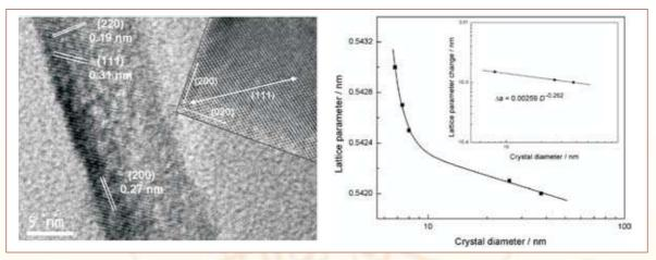
HR-TEM image of segment of a nanorod with a cuboidal  $CeO_2$  crystal in the inset (left). Semilog profile of lattice parameters against the size of  $CeO_2$  crystals of different shapes (right). Inset is the log-log plot of change in lattice parameters as a function of crystal diameter.
