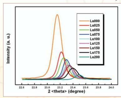
Systematic increase in peak position and decrease in peak intensity of an XRD peak (008) of Lu doped (Bi, Pb)-2212 superconductor with respect to Lu content showing a contraction of c-lattice parameter and decrease of texture.
