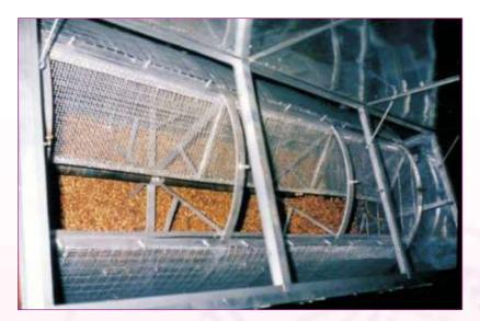
Inner cylindrical chamber of ground nut drier
