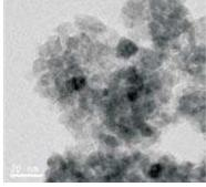
TEM image of 30% silica doped TiO\_2 calcined at 700°C
