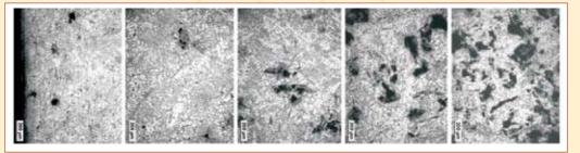
Microstructures of Graphite and primary silicon reinforced hybrid FGM from outer edge of the casting
