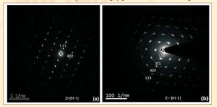
Selected area electron diffraction (SAED) patterns showed highly ordered diffraction maxima with characteristic weak diffraction spots of the pyrochlore structure for (a)  $Ca_{0.6}$  7Y<sub>1.33</sub> $Tr_{0.33}O_{7}$  (C2YZT2) and bright diffraction maxima arranged in a ring pattern of the fluorite structure for (b)  $Ca_{0.29}$  7Y<sub>1.71</sub> $Zr_{1.71}$  $Ta_{0.29}O_{7}$  (CY6Z6T).
