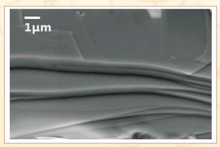
SEM image of clean large flaky grains of Lu doped (Bi, Pb)-2212 superconductor
