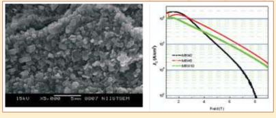
SEM image of pure MgB<sub>2</sub> superconductor showing faceted hexagonal grains (left) and variation of critical current density of pure (MRH0) and burned rice husk doped (MRH5 and MRH10) MgB<sub>2</sub> samples with respect to magnetic field at 5 K. The doped samples exhibit excellent field withstanding capability (right).
