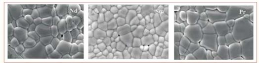
Typical sintered microstructures of PbRETiTaO<sub>7</sub> ceramics.
