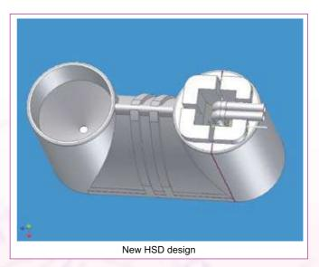
from a flat in NIIST Staff Quarters. There was difficulty in start-up and acidification if combined black and grey water were treated in the digester chamber. It was found that better treatment efficiency is obtained by separate black water treatment in digester while grey water is directly sent to biofilm tank. Mathematical modeling studies supported the observation.
