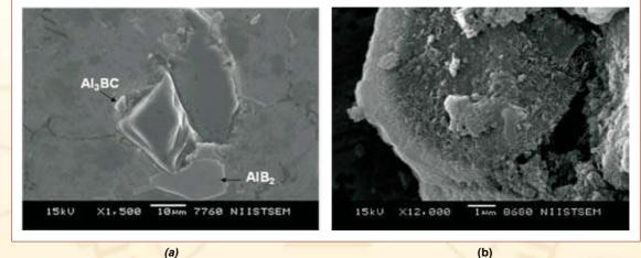
SEM micrographs of (a) Al(6061\_-B4C MMC and (b) extracted B4C particle showing interfacial reaction products on the surface.
