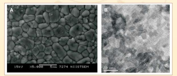
A) SEM image of LaPO<sub>4</sub>-20% Y<sub>2</sub>O<sub>3</sub> sintered disc at 1600°C B) TEM image of LaPO<sub>4</sub>-20% Y<sub>2</sub>O<sub>3</sub> powder heated at 500°C.
